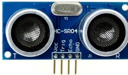
Gambar 5. Sensor Ultrasonik HC-SR04 [15]
