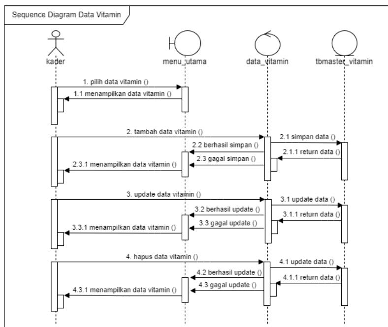
Gambar 3.17 Sequence Diagram Data Vitamin
