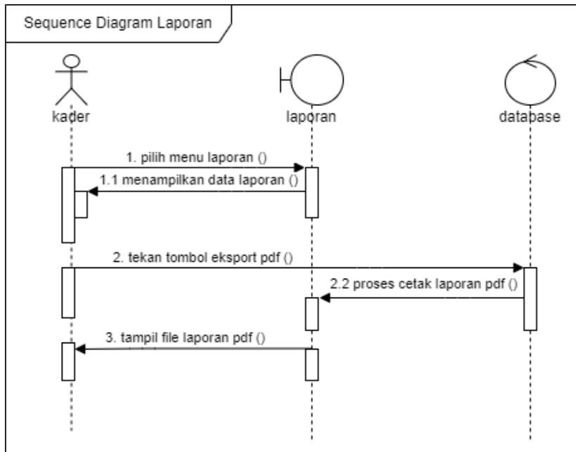
Gambar 3.19 Sequence Diagram Laporan
