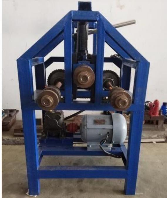
Gambar 4. Gambar rol bending
