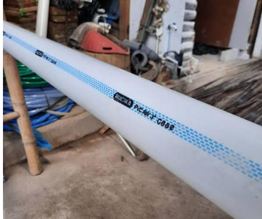
Pipa inlet 2 inch
