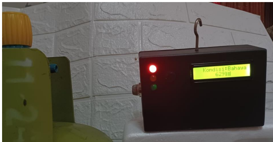
Gambar 4. 5 Alat mendeteksi kebocoran gas LPG
