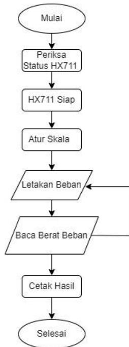
Gambar 13 Diagram Alur Kalibrasi
