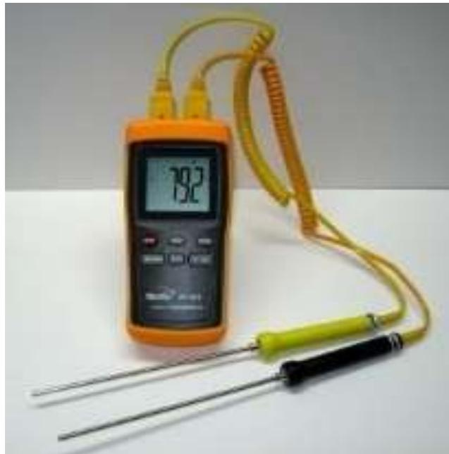
Gambar 2. 10 Thermocouple
