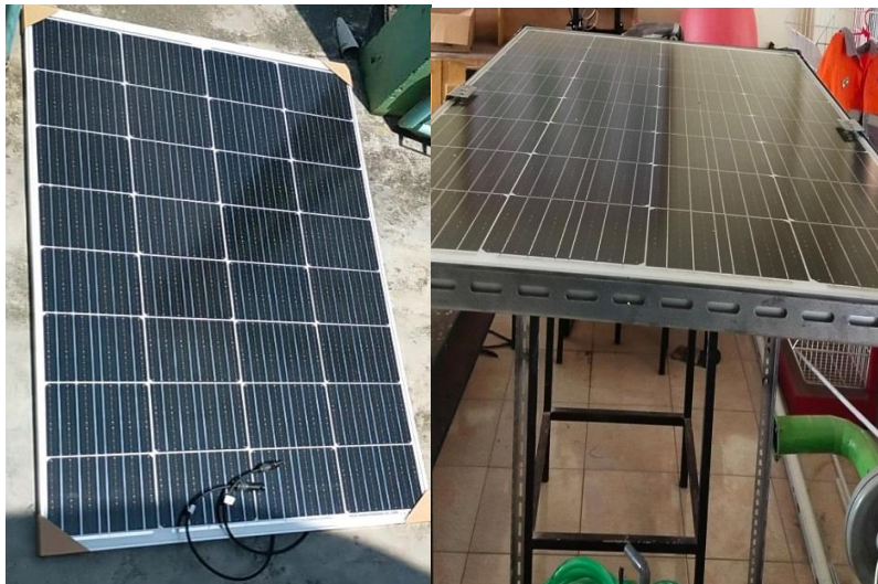
Gambar 4.4 Panel surya Monocrystalline 200 WP
