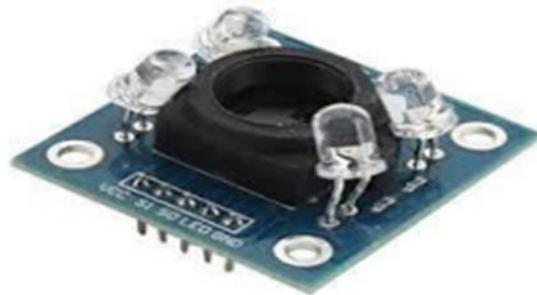
Gambar 2.3 .Sensor Warna TCS 2300.
