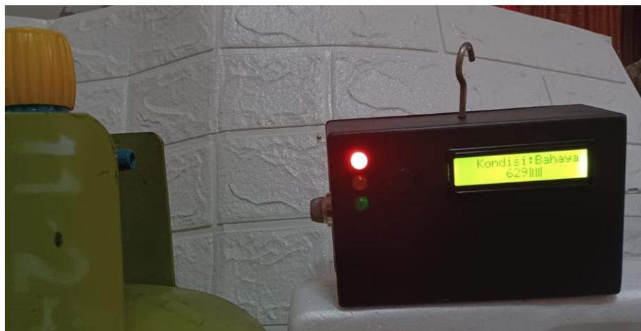
**Gambar 4. 5** Alat mendeteksi kebocoran gas LPG
